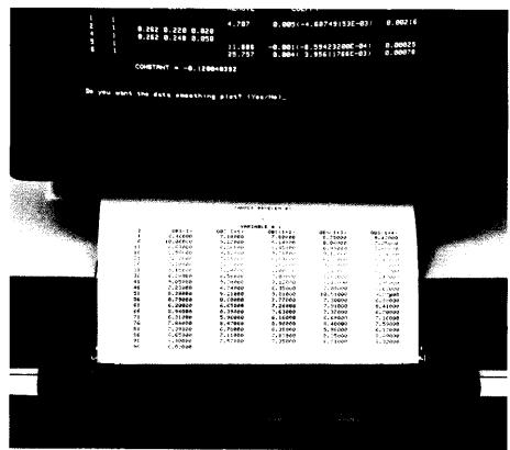
The low-cost, 80-column line printer, offered as either a factory- or field-installable option, fits directly into the system, beneath the CRT.
