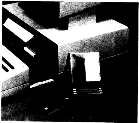
The System 45 allows the addition of up to eight read-only memories (ROMs) that can fit into drawers found on the sides of the machine.
